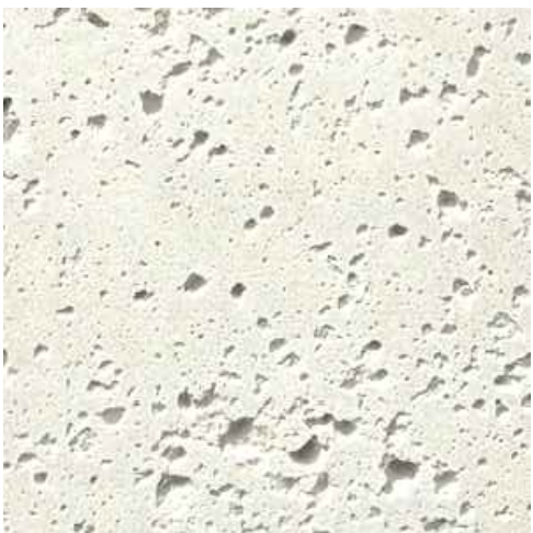
② PRECAST CONCRETE PANELS TEXTURE FINISH
