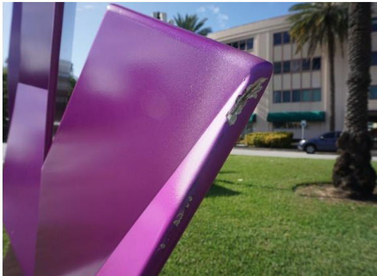
Figure 5. Gouge and coating loss on the top edge of the bottom prism (photo by EverGreene, February 2021).
