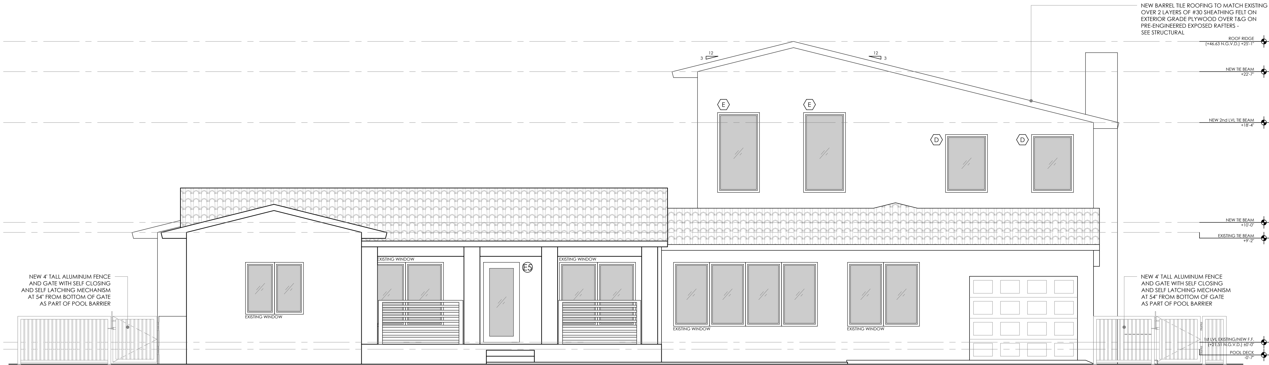
1 NEW NORTH ELEVATION SCALE: 1/4" = 1'-0"
