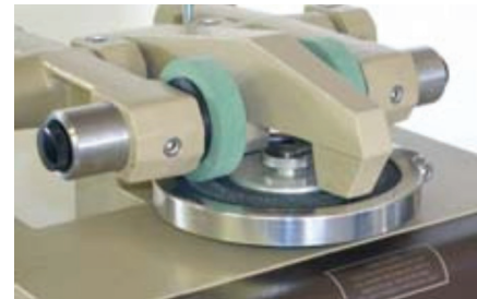
The Taber Rotary Platform Abraser
