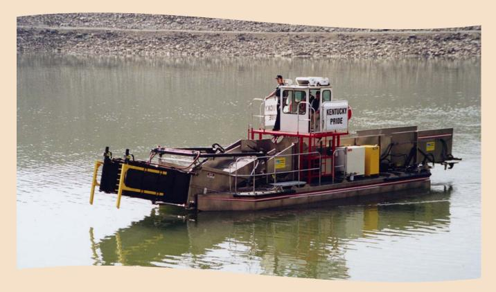
Standard Trash Hunters feature an elevated pilot house located over the storage hold for maximum visibility. An optional low profile configuration is also available if clearing low-hanging overhead obstructions are a concern.
