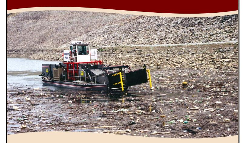
Trash Hunters are the ideal tool for removing floatable debris from harbors, rivers and other waterways plagued with unsightly hazards. The Trash Hunters easily retrieve a wide variety of manmade and naturally occurring debris including floating litter, old tires, timber, branches and logs.
