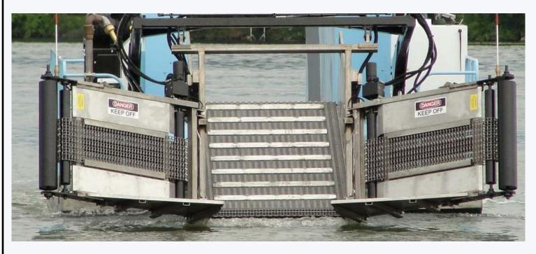
The **Combination Wings** have both heavy duty conveyor mesh and solid steel construction. They provide the strength to collect heavier materials like tree limbs, and include conveyorized mesh at the water line to aid in the collection of lightweight floatables. The conveyor belting is designed for quick change-out and repair when necessary.
