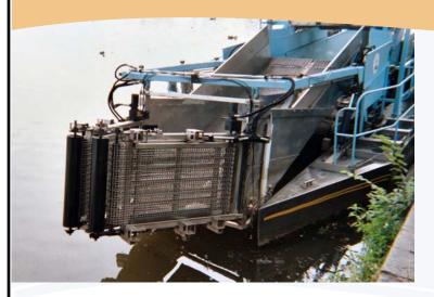
The standard collection wing is a **Solid Steel** design that can tolerate abuse from heavy debris like logs and trees (*shown above*).
