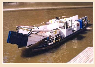
Complete instrumentation and hydrostatic hydraulics make handling the skimmer a simple task for a single operator. Twin hydraulic propellers - the most efficient propulsion system available for both speed and performance - power the trash collectors.
