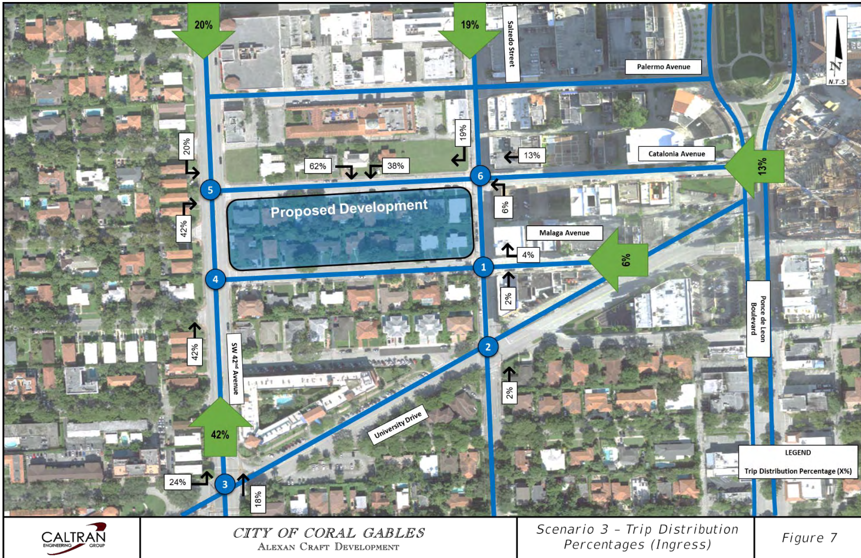
Figure 7: Peak Hour Development Trip Distribution (Ingress)
