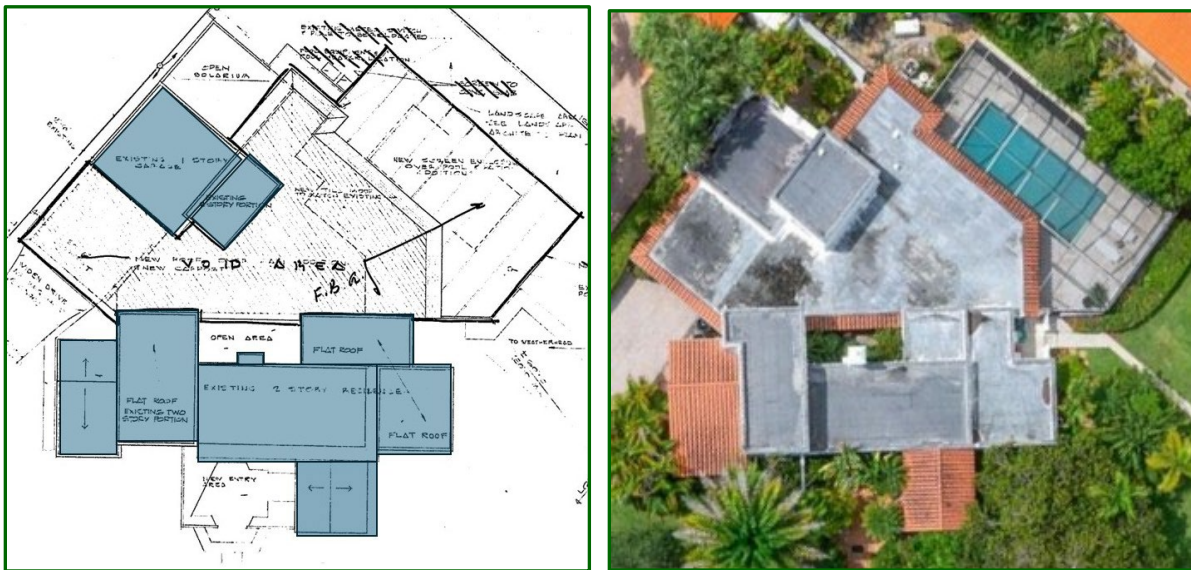
Figures 33: Footprint of 1923 Structures and 1969 Addition
