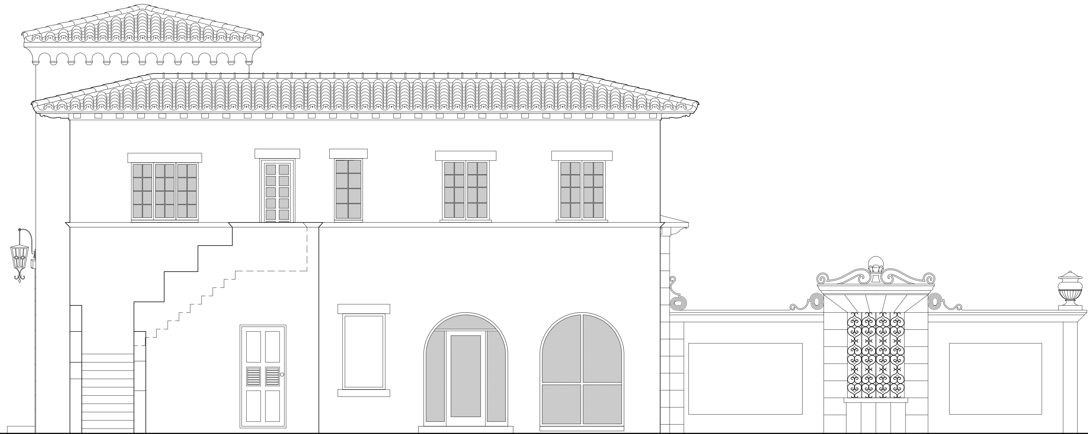
SOUTH ELEVATION - EXISTING SCALE: 1/4" = 1'-0"
