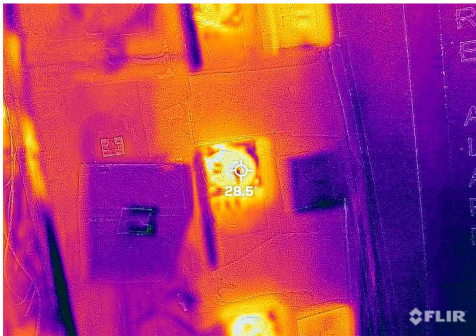
Item 63: Time Clock at 28.5 Degrees Celsius (delta 5.5C)
