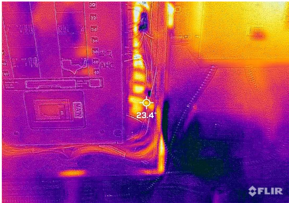
Item 72: Panel 3AC at 23.4 Degrees Celsius (delta 3.4C)
