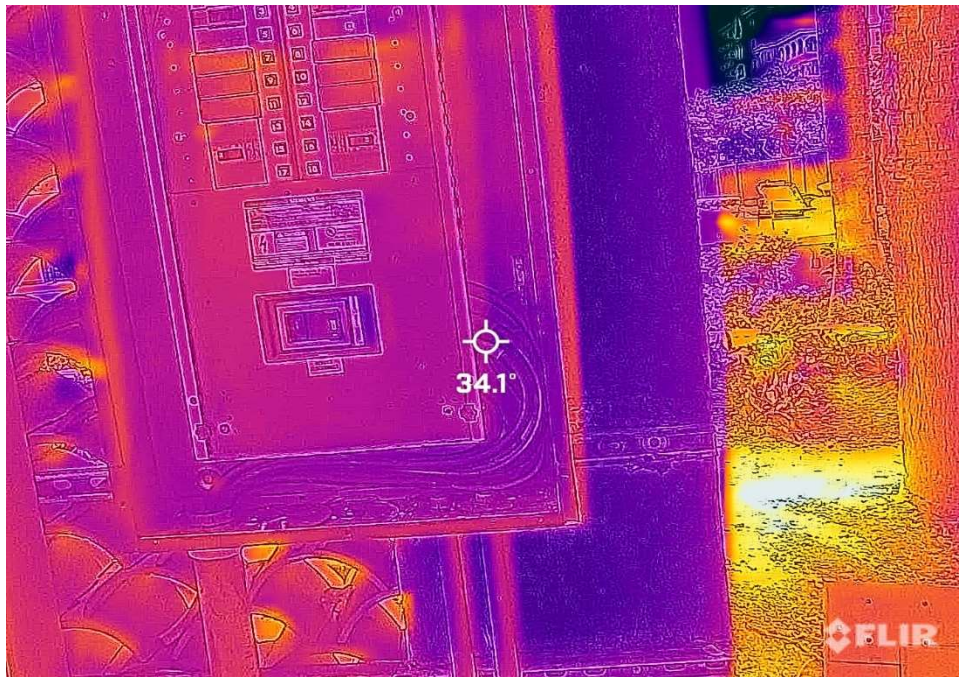
Item 53: Panel 1AC at 34.1 Degrees Celsius (delta 4.1C)
