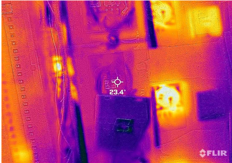
Item 60: Relay at 23.4 Degrees Celsius (delta 0.4C)
