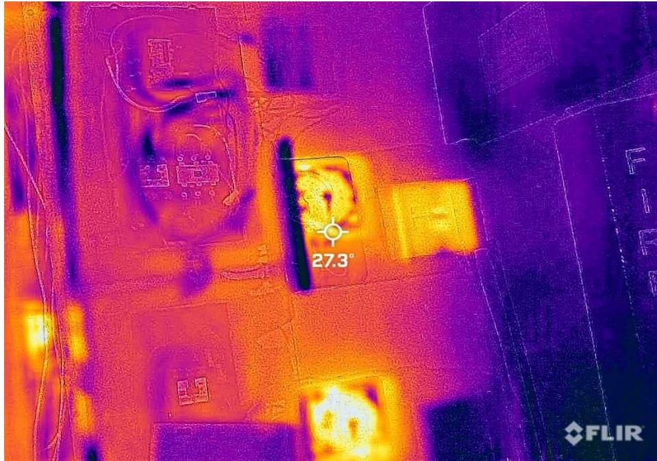
Item 64: Time Clock at 27.3 Degrees Celsius (delta 4.3C)
