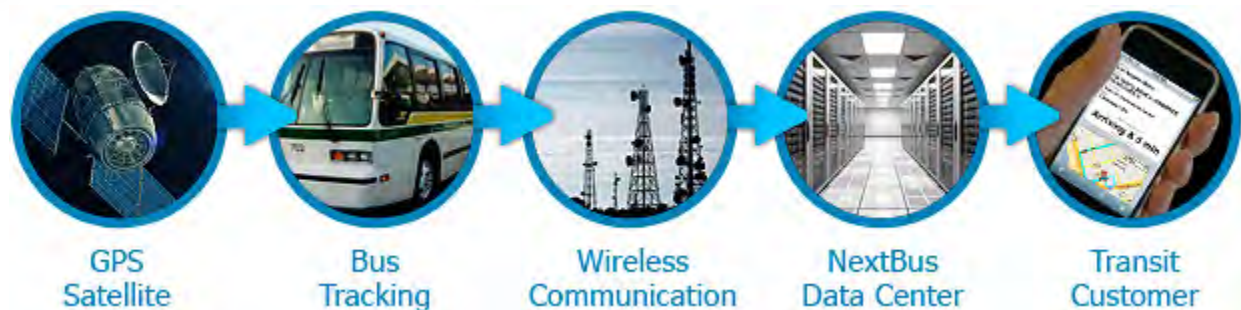
Figure 7-3 - NextBus Passenger Information System Information Flow
