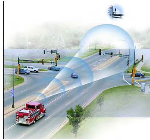
Figure 7-4 - Representation of Traffic Signal Priority System
