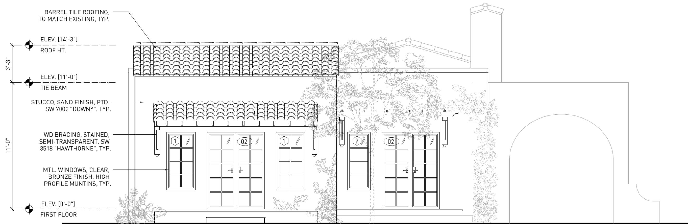
4 PROPOSED REAR (NORTH) ELEVATION 1/4" = 1'-0"
