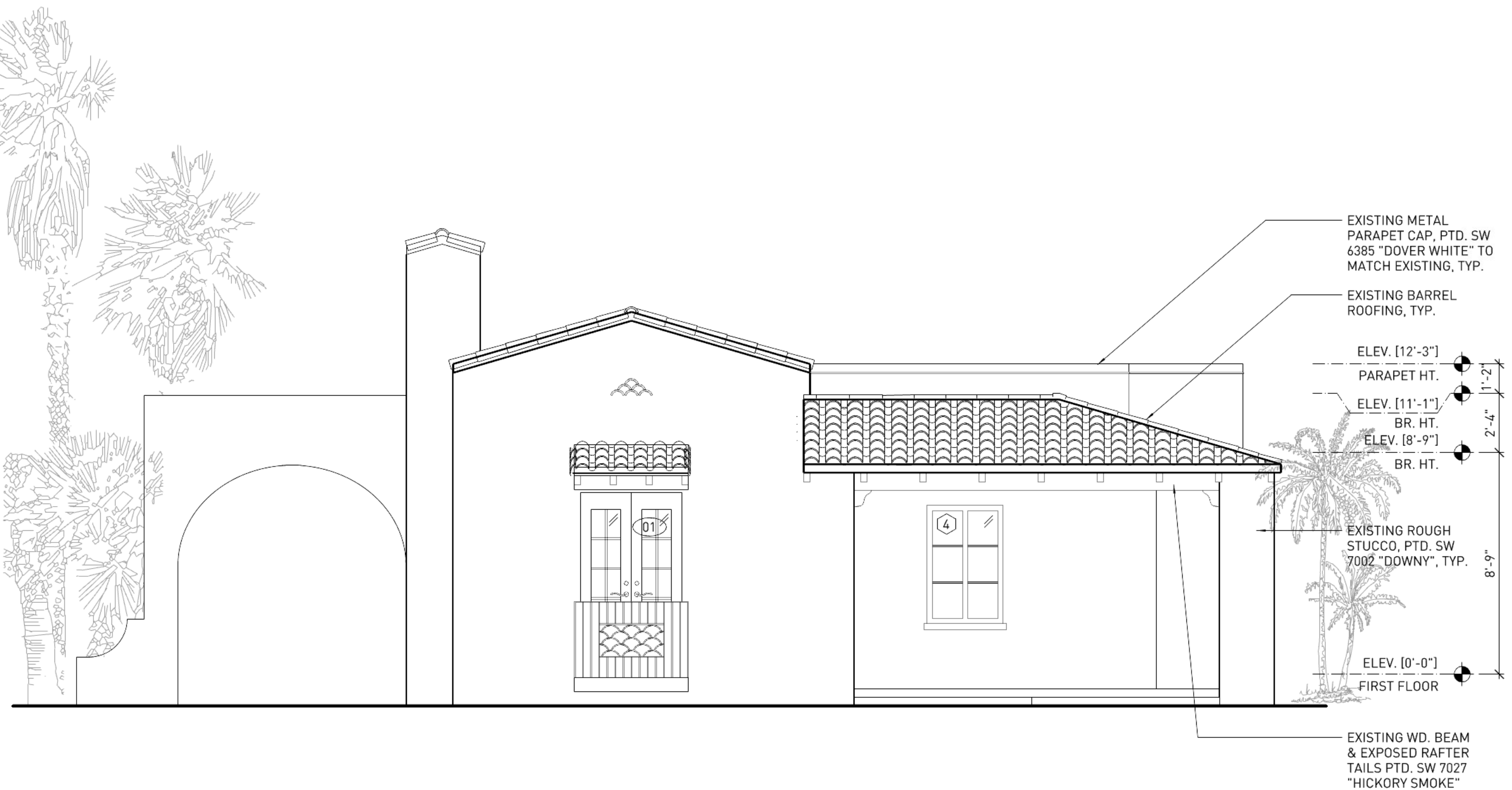
2 PROPOSED FRONT (SOUTH) ELEVATION 1/4" = 1'-0"
