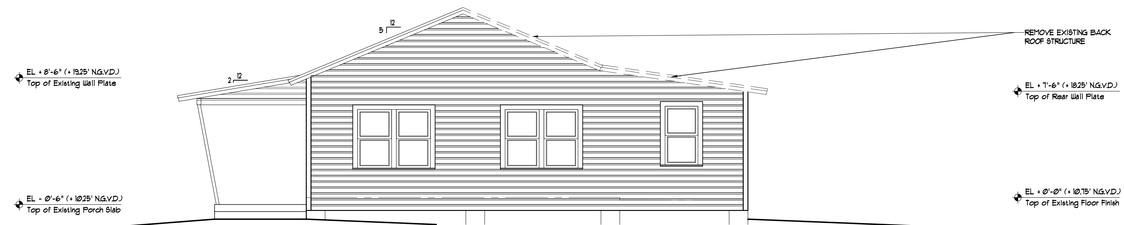
Demolition West Elevation
