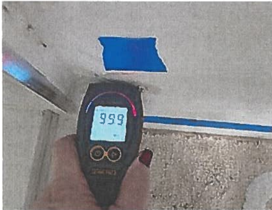
Elevated Moisture Content Detected with A Moisture Meter
