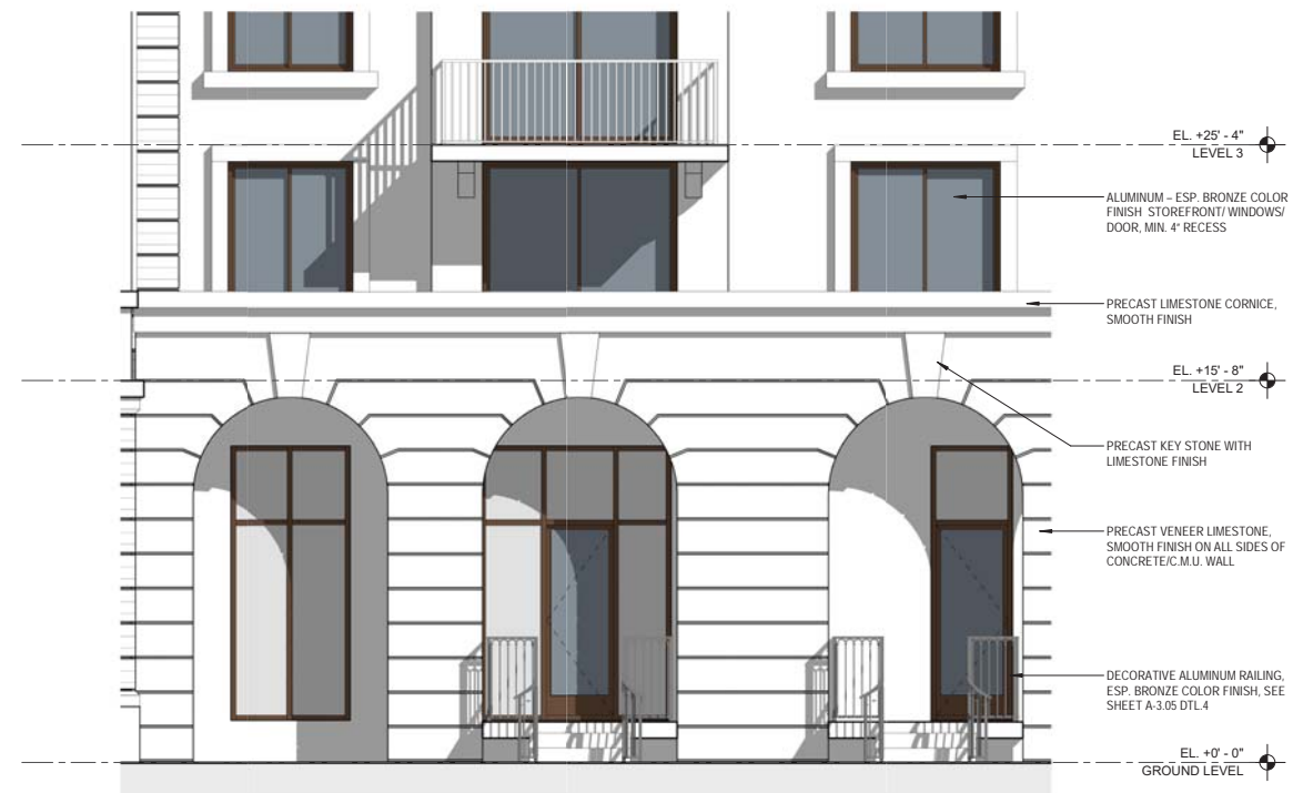
ENLARGED PARTIAL STOOP ELEVATION SCALE: 1/4" = 1'-0"
