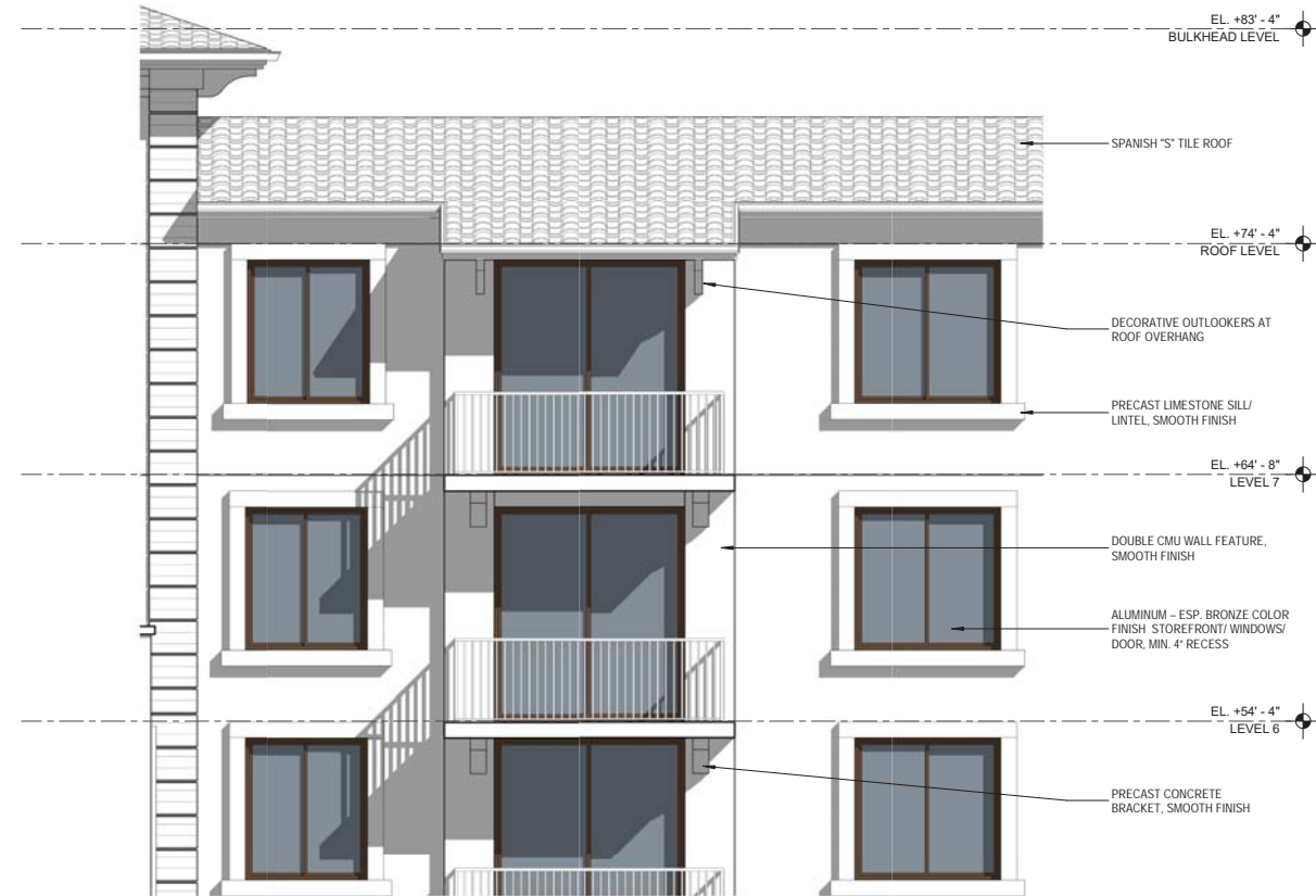
ENLARGED PARTIAL BALCONY ELEVATION SCALE: 1/4" = 1'-0"
