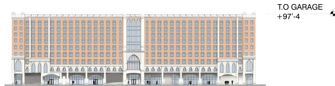
G1 - 9 LEVEL PODIUM WITH 8 LEVELS OF PARKING
