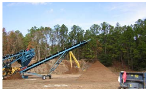
Excavation, Sifting, and Stockpiling of lead
