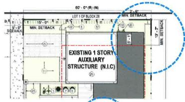
2)- Side Street Setback facing Pizarro Street: The New Pool, Its equipment, Deck, and The 4' high Wall (for visual screening), all encroach into the 15" required setback. Variance = allow for 8'-6 3/4" encroachment beyond the 15' setback requirement.
