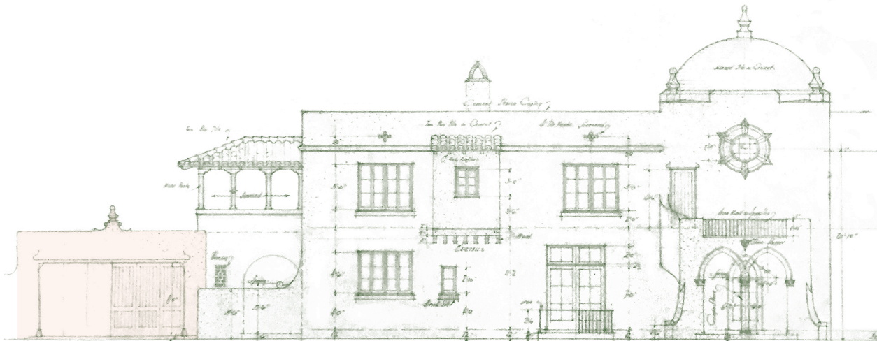
Garage Doors set back from Front Facade
