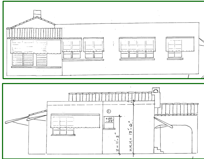
Figures 25: South Side [top] & Rear [bottom] Facades with Hurricane Awnings over Original Width of Sleeping Porch Openings Permit #5050573, 2005
