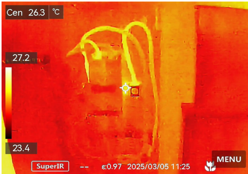
7.3.1 A C Disconnect – Delta T 1.3 (C°)
