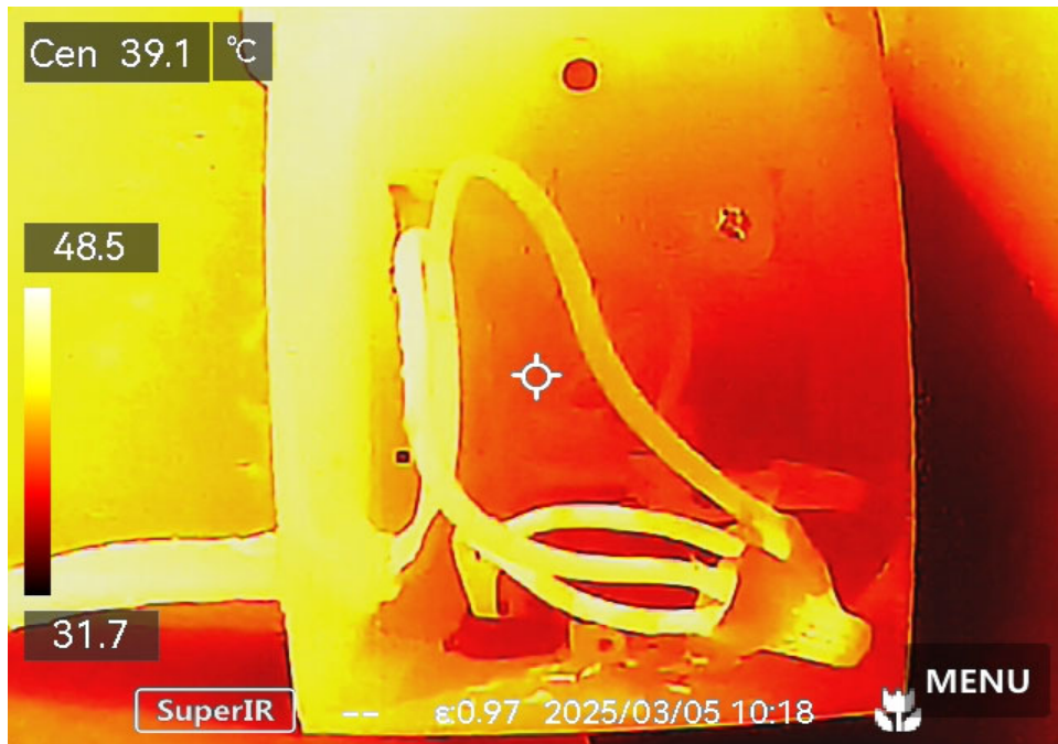
7.7.1 A C Disconnect – Delta T 10.1 (C)
