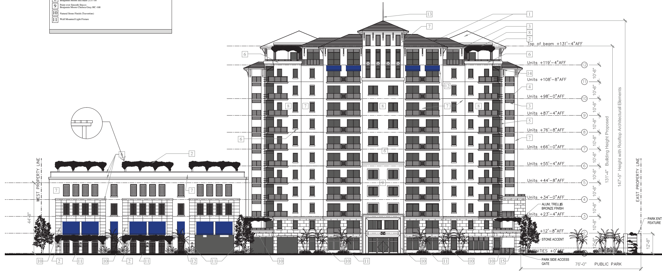
ELEVATION (SOUTH) SCALE: 1/16" = 1'-0"
