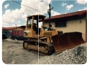
CAT D3G Dozer
