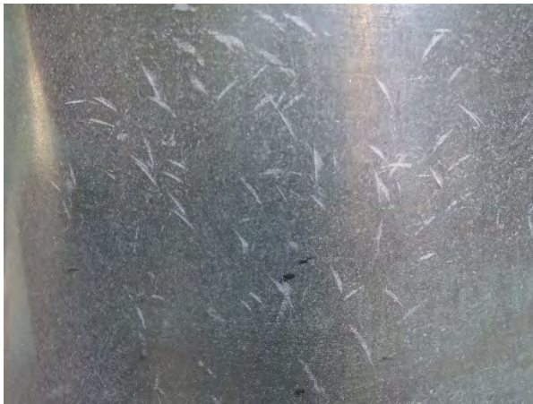
(Left) Linear abrasions with a silvery appearance on the south side of the bell. (Right) Weathered lacquer coating on the dedication plaque.
