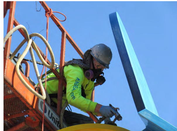
Applying the clear coat with a roller (left) and an HVLP sprayer (right).
