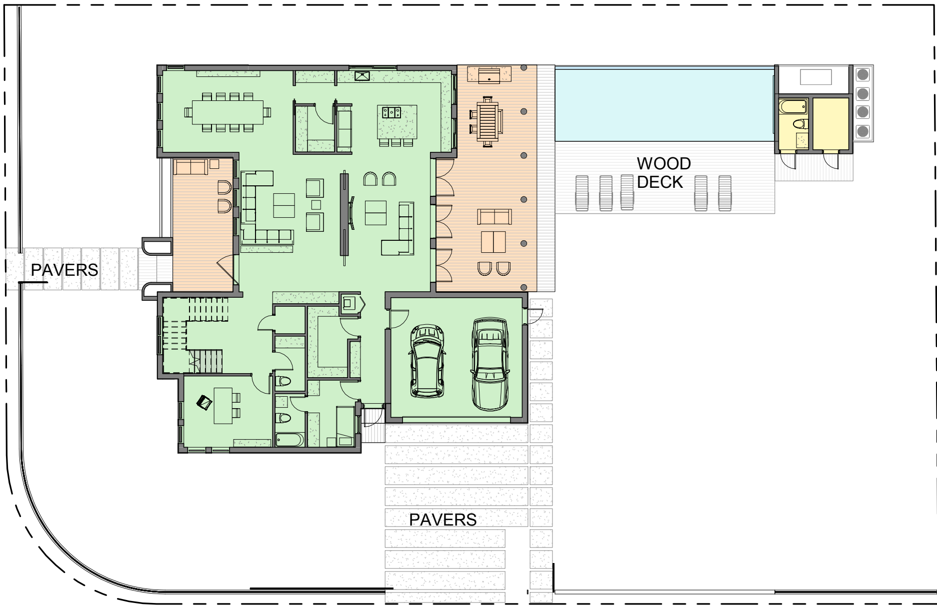
4 GROUND FLOOR PLAN - LOT COVERAGE DIAGRAM 1/16" = 1'-0"
