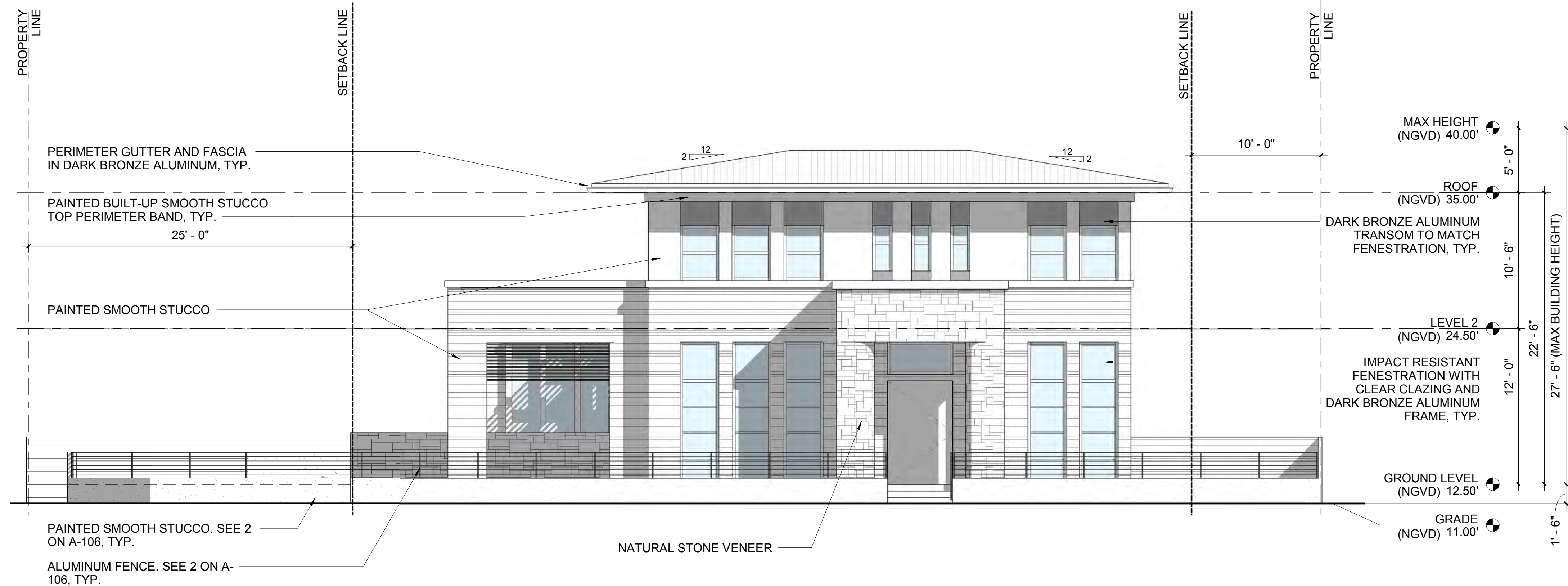
2 SOUTH ELEVATION WITH FENCE 3/16" = 1'-0"
