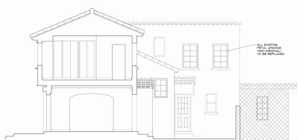
Existing Building Section / Elevation facing East Scale : 1/4" = 1'-0"
