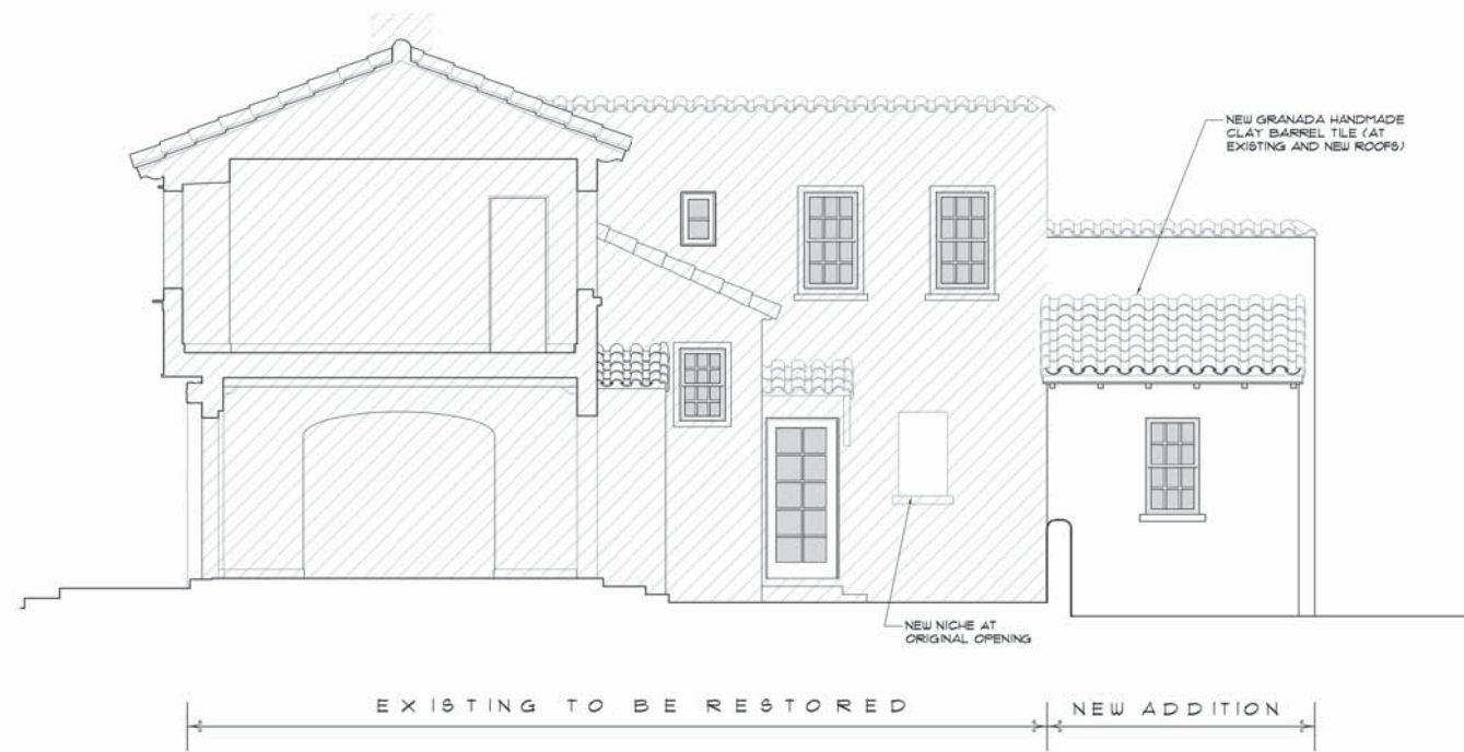
Proposed Building Section / Elevation facing East Scale : 1/4" = 1'-0"
