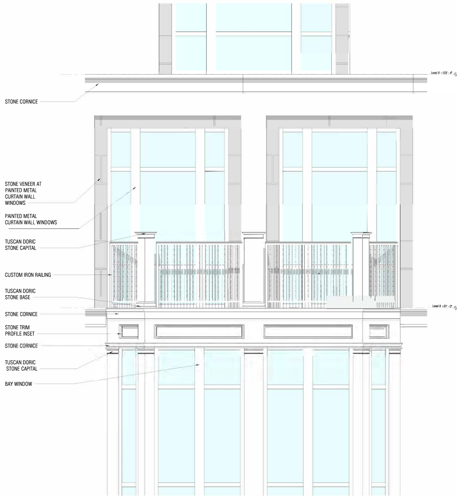
1) Bay Window to Storefront Elevation Scale: 3/4" = 1'-0"
