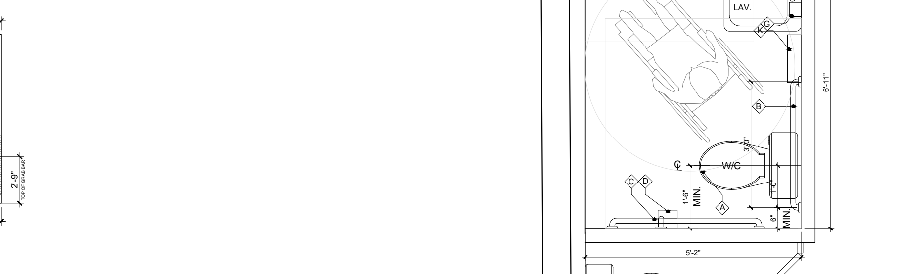
TOILET ACCESSIBILITY NOTES: 1. DOORS TO THE H.C. TOILET ROOMS SHALL BE 30" WIDE. 2. PROVIDE DOOR HARDWARE - PRIVACY TYPE LOCKSET WITH LEVER TYPE ACCESSIBILITY APPROVED HARDWARE. DOORS SHALL BE EQUIPPED WITH ACCESSIBILITY APPROVED CLOSER AS PER SECTION (404.2.7) OF THE FLORIDA BUILDING CODE, ACCESSIBILITY 2017 ED. 3. GRAB BARS (STAINLESS STEEL) SHALL HAVE A 1 1/2" MIN. AND 2 INCH MAX. O.D. AND SET 1 1/2" AWAY FROM THE WALL AND 33" 36" ABOVE THE FINISHED FLOOR. SIDE GRAB BAR SHALL BE 42" LONG. GRAB BAR BEHIND TOILET SHALL BE 36" LONG. AS PER SECTION (609.4) AND FIGURE (609.3) OF THE FLORIDA BUILDING DEPARTMENT, ACCESSIBILITY 2017 ED.
