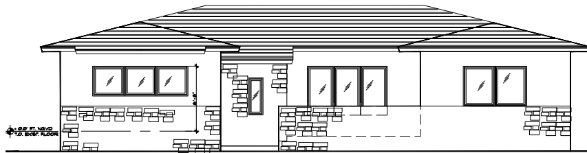
FRONT ELEVATION-SOUTH VIEW-EXISTING 1/4" = 1'-0"
