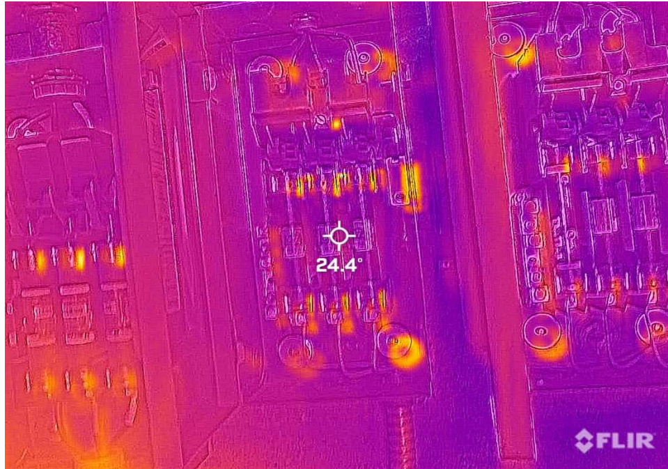
Item 32: Air Comp Disconnect at 24.4 Degrees Celsius (zero delta)
