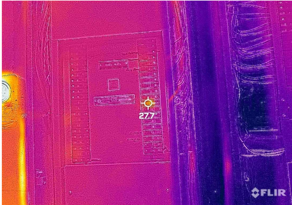
Item 73: Panel N12L at 27.7 Degrees Celsius (delta 4.7C)
