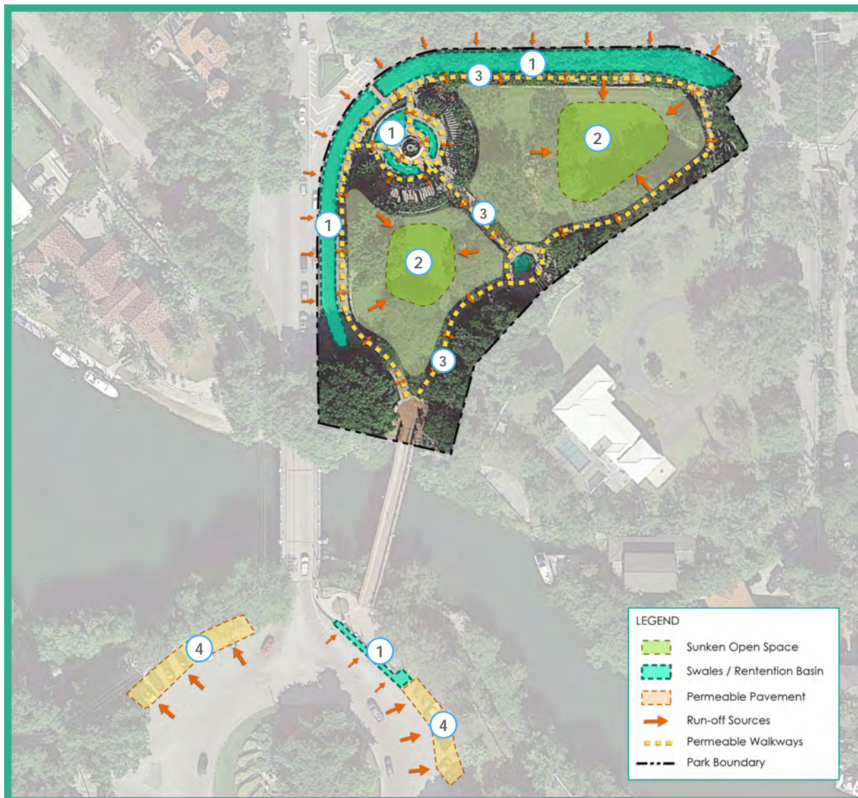
Figure 4-3: Potential Neighborhood Drainage at Ingraham Park
