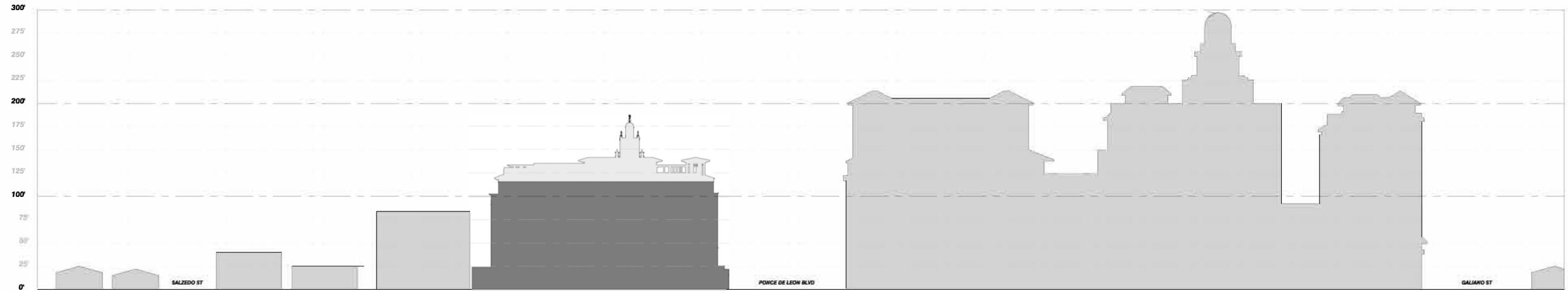
250 CATALONIA 80' PONCE PARK RESIDENCES 115'-0" ROOF HEIGHT 178'-10" DOME HEIGHT 186'-6" ARCH (STATUE) HEIGHT THE PLAZA 218'-0" ROOF HEIGHT 297'-0" ARCH HEIGHT
